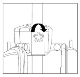
Step 4: When start using the heater, just holding the little handle by the end of the heater and push up.
