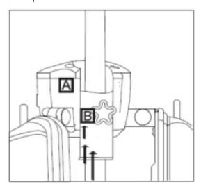
Step 3: Turn the Fixation Screw until the Mounting Part A is fixed on the pole
