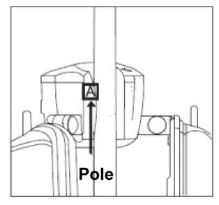
Step 2: Slip the Mounting Part B and fit it to the Mounting Part A from the bottom up.
